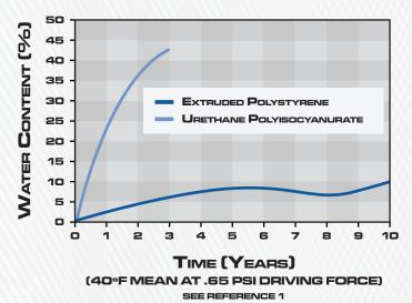
As you can see in the following graph, polyurethane loses over 75% of its R-value in five years and extruded polystyrene loses only 25% of its R-value. Therefore, extruded polystyrene's performance, in actual walk-in conditions when moisture is considered, is over three times that of polyurethane.
