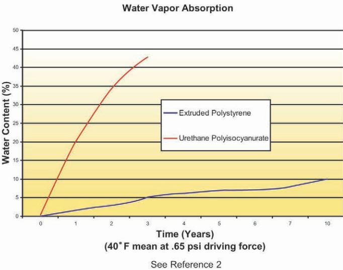
As you can see in the following graph, polyurethane loses over 75% of its R-value in five years and extruded polystyrene loses only 25% of its R-value. Therefore, extruded polystyrene's performance, in actual walk-in conditions when moisture is considered, is over three times as good as polyurethane.
