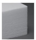
FOAMULAR extruded polystyrene insulation is a closed-cell insulation made using the exclusive Owens Corning HYDROVAC® manufacturing process. FOAMULAR insulation's resistance to water absorption and water vapor transmission allows it to maintain a high thermal resistance through the life of the walk-in cooler or freezer unit. FOAMULAR is hydrophobic; the closed-
