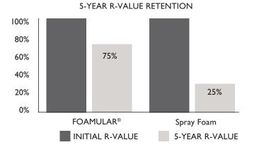
Testing conducted by the U.S. Army Corps of Engineers Cold Regions Research and Engineering Laboratory
