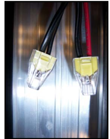
2.6 Connect wires from LED fixture to Black and Red wires from wire assy. Using Wago connector Part# 773-162 or other approved connector as shown.
