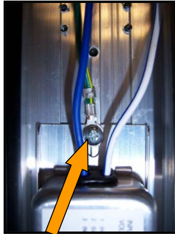
3.2 Attach ground wire from frame power harness as shown.
