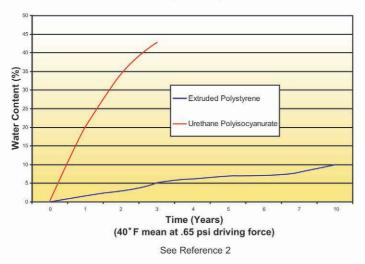
As you can see in the following graph, polyurethane loses over 75% of it's R-value in five years and extruded polystyrene loses only 25% of its R-value. Therefore, extruded polystyrene's performance, in actual walk-in conditions when moisture is considered, is over three times as good as polyurethane.
